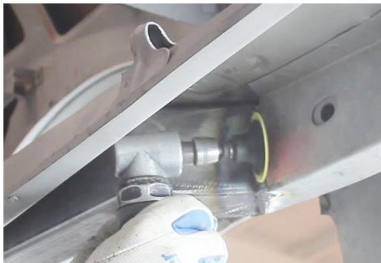
Figure 23 – Weld Inside Frame Rail Doubler Plate
