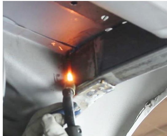
Figure 22 – Weld-In DSE Frame Rail Section
