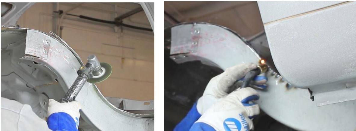
Figure 20 – Cut & Weld Sheet Metal Layers
