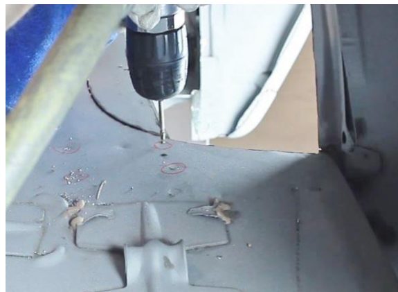
Figure 15 - Drill-Out Spot Welds
