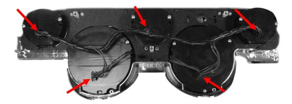
11. This system comes with the option to use two sets of turn signals and the high beam located in the faceplate of your new RTX display, and arrows/high beam indicator in your vehicle's stock locations. To use the new faceplate indicators, follow the wiring instructions for the turn signals found in the main RTX manual.
