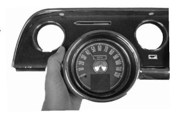
5b. Use the provided 2" screws to mount the gauges in place. Do not fully tighten; the holes are slotted to allow minor adjustments to perfectly align each gauge. For the Speedometer and Tachometer, use the two provided brackets at the bottom slots as shown in blue arrows. Once aligned, finish tightening the 12 screws.
