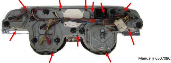
2. Remove the stock gauges, separator plates, and lenses from the bezel.
