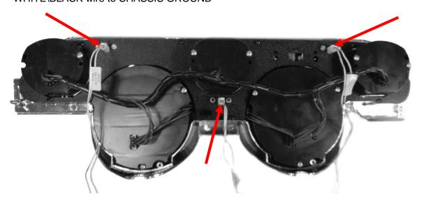
12. Connect the provided display harness and the buzzer (optional for audio feedback) to the back of the RTX system.
