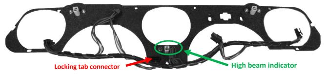
9. Lay the ABS panel over the back of the gauge cluster with the smooth side down and slip the wiper arm through the appropriate opening in the bezel. Use the seven (7) supplied ½" black screws to mount the panel to the back of the bezel. Ensure harness wires are not pinched.
