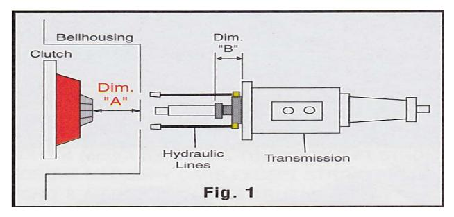
To Determine "Dimension A": With the bell housing, flywheel, disc and pressure plate bolted to the engine, measure the distance from the rear surface of the bell housing to the top of the release fingers on the pressure plate. If this dimension measures less than 3" you should use a "Bolt-On" style hydraulic throw out bearing assembly. If this dimension measures greater than 3" you should use a Slip-On style hydraulic throw out bearing assembly.
