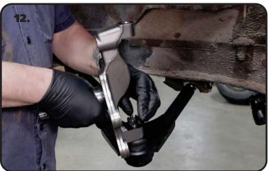
**12.** Install the spindle on the lower ball joint pin. Torque the ball joint castle nut to 65 ftlbs and tighten to align the cotter pin holes. Install the cotter pin in the ball joint pin hole and bend the ends of the cotter pin to hold it in place. Install the grease zerk supplied with the ball joint.
