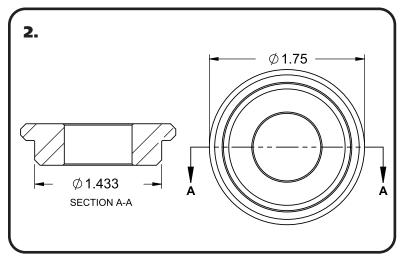
**2.** This kit includes a t-bushing for the strut rod bushing factory hole.
