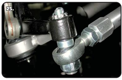
**25.** Install a 5/8"-18 mechanical locking nut. Torque to 45 ftlbs.
