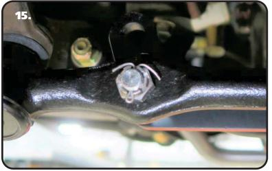
**15.** Torque the nuts to 35 ftlbs and tighten as needed to align cotter pin. Install cotter pin and bend the ends.
