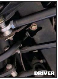
**5.** The new suspension brace bolts in place of the original brace. Install a 1/2"split lock washer & 1/2" flat washer on each of (2) 1/2"-13 x 1" bolt. Position the crossmember brace at the factory location, behind the lower control arm mount. Align the mounting holes of the crossmember with the mounting holes in the frame rails. Install a bolt/washer in each of the mounting holes. Torque the crossmember hardware to 50 ftlbs.
