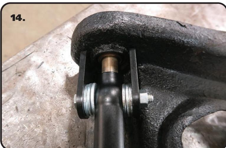
**14.** Bolt the Short Cross Shaft Tabs to the cross shaft using (1) 5/16"-18 x 2 1/4" Hex Bolt, (6) 3/8" Flat Washers & (1) 5/16" Hex Nut. The Tabs will be bolted to the cross shaft using the cross shaft mounting holes with (3) 3/8" Flat Washers between each Tab and The Cross Shaft. Place a Tab on each side of the cross shaft with the flat side against the control arm. Tighten the 5/16" bolt/nut with the flats squarely against the control arm.
