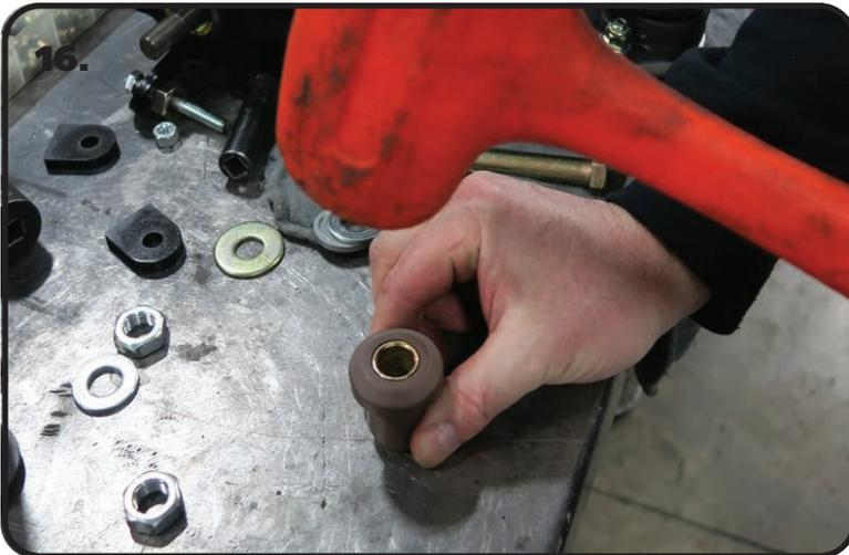
16. Install the 9/16" ID inner sleeve into the delrin bushing. You can tap it in with a hammer. Be careful to not distort the edge of the bushing with the hammer. Once the Inner Sleeve is installed, start the assembly into the outer shell installed in the arm. It can be pushed in partially by hand
