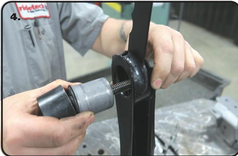
**4.** Using a wrench on each hex, tighten the nut. The bushing should start pushing out of the arm. Keep tightening the nut, pushing the bushing out of the arm. Once the bushing pops out of the arm, remove the tool leaving the support in place to install the Delrin Bushing setup.
