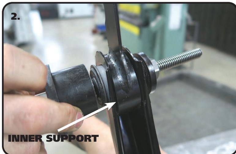
2. Start by sticking the Inner Arm Support in the arm with the "C" shape cradling the bushing. This support keeps the control arm from deforming while removing and installing the bushings.
