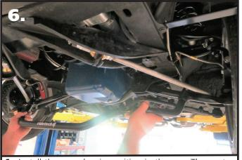
**6.** Install the sway bar in position in the car. The center of the bar should be to the front of the car. The outer arms of the sway bar will bend upward. Use **Picture 6** as a reference.
