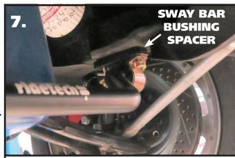
**7.** Install a 3/8" flat washer on each of the (4) 3/8" x 1 1/2" bolts. The sway bar bushing spacer will be installed between the sway bar bushing and frame. Push the bar up to the frame, installing the spacer in place. Hold it in position and install (2) bolt/washers in each side. Install a 3/8" flat washer & 3/8" nylok nut on the bolts and snug the hardware.
