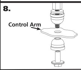
**8.** Install the End Links using **Diagram 8** as a reference. Tighten the end link barrel nut until it is flush with the end of the bolt, and then tighten it 2 more complete rounds.
