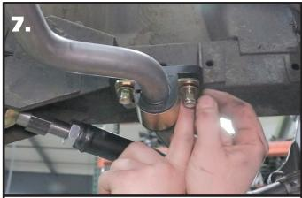
7. Install the sway bar in position in the car. The center of the bar should be to the front of the car. The outer arms of the sway bar will bend upward. Install a 3/8" flat washer on (4) 3/8"-16 x 1 1/4" hex bolts. A bolt/washer will go in each of the 4 mounting holes. With the bolt/washers installed, install a 3/8" flat washer on the threads followed by a 3/8"-16 nylok nut. Do **NOT** completely tighten the hardware. It will be left partially loose until the end links are installed.
