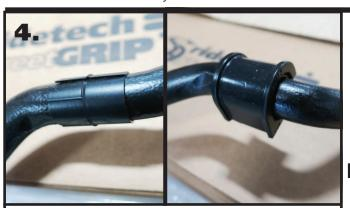
**4.** Open the delrin liner at the split and slip it over the swaybar. Position it in the area that the bushing will ride based on the location of the stock swaybar. Do this on both ends of the swaybar. Next, open the swaybar Bushing at the split and slide it **OVER** the delrin liner. Do this on both delrin liners.
