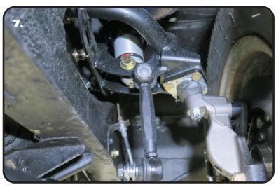
7. Remove the nut from the top end link. Insert the stud of the end link in the tab of the upper control arm with the stud pointing to the rear of the car. The lower stud should be pointing toward the engine. Install the nut on the stud of the end link and torque to 37 ftlbs. Repeat on the second side.
