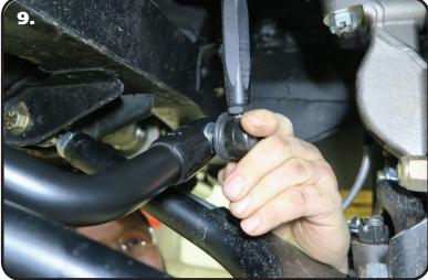
**9.** Insert the 90 degree end link/t-bushing into the swaybar end with the threads pointing toward the engine.
