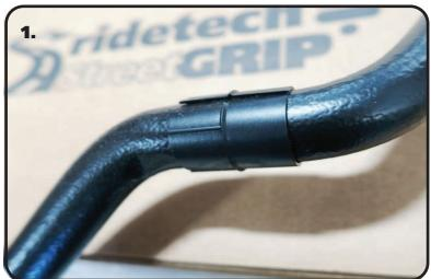
**1.** The delrin liner is split on one side to ease installation. Install a liner on each side of the swaybar in the approximate location they will need to be when installing the sway bar on the car.
