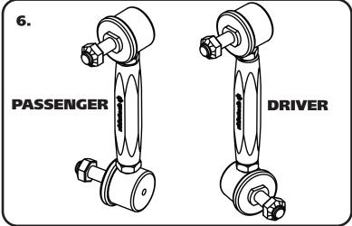
**6.** The driver and passenger sway bar linkages are clocked opposite of each other. With the top stud pointing toward you, the stud on the lower should be pointing to the right for the driver side, to the left for the passenger side. Using **Diagram 6** as a reference, set the linkage to 6" center to center. Snug the jam nuts against the center adapter.
