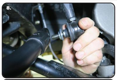
**8.** Remove the nut from the bottom end link. Install a t-bushing on the lower 90 degree end link. The t-bushings are installed with the large diameter against the shoulder of the end link.
