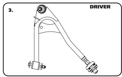
**3.** The control arms are marked "D" for Driver and "P" for Passenger. The ball joint pin points down and the sway bar mount is on the front side of the arm.
