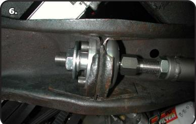
**6.** Slide the stud through the bearing, then slide the aluminum spacer over the stud with the larger end toward the front of the car. Secure the assembly with a <sup>3</sup>/<sub>4</sub>" Nylok Nut and flat washer. Use **Images 6 & 7** as a guide.
