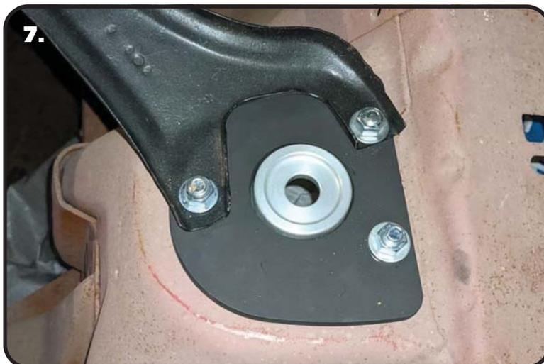
7. Install the export brace on the bolts sticking through the top plate. Install a 3/8" SAE flat washer & 3/8"-16 nylok nut on the threads of each of the bolts. Torque the nylok nuts to 15 ft-lbs.
