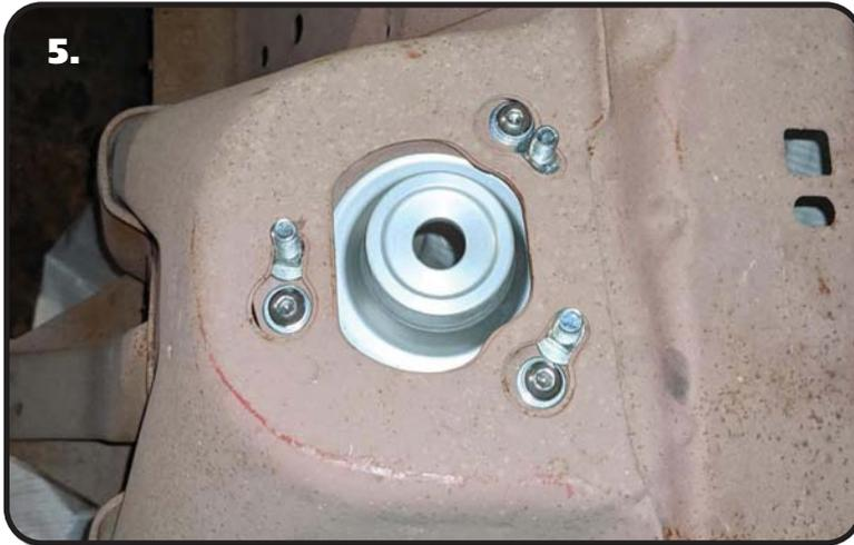
5. Install a 5/16" split lock washer & 5/16" SAE flat washer on each of (3) 5/16"-18 x 1" button head cap screws. Apply red loctite to the threads of each of the bolts. Hold the lower mount in position and thread the mounting bolts into the (3) mounting holes. Torque the bolts to 13 ft-lbs.
