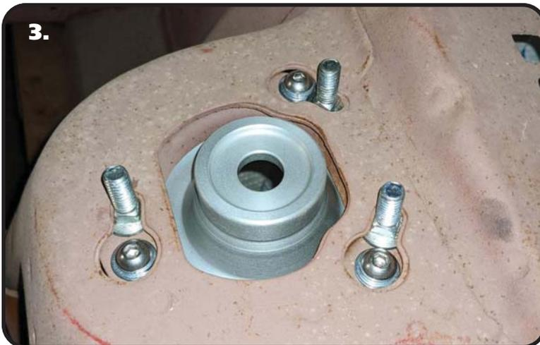
3. Slip the 3/8"-16 x 1" carriage bolts into the slots of the shock tower before bolting in the aluminum mount. **You can NOT slip the carriage bolts in with the upper mount bolted in place.**
