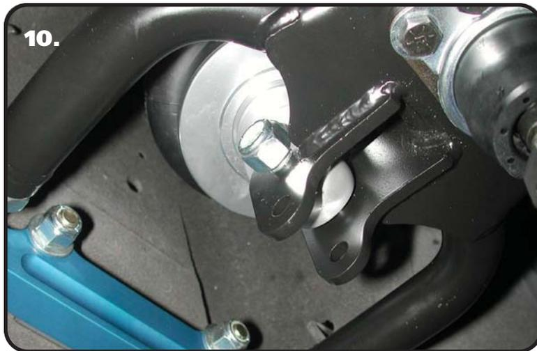
**10.** Install the a Bearing Spacer in each side of the Bearing. The SMALL part of the spacer inserts into the Inside Diameter of the shock bearing. Raise the lower arm up to the CoilOver and bolt them together using the 1/2" x 2 1/4", & Nylok Nuts supplied with the StrongArms. Torque to 50 ftlbs.
