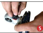
Once the knob is removed slide a Delrin washer over the eyelet. Next, slide the upper spring mount (803-00-199) over eyelet as seen in figure 4.
