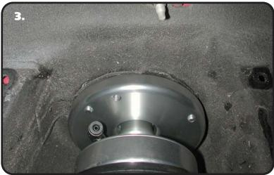
**3.** Hold the Aluminum Upper Mount agianst the bottom of the shock tower lining up the threaded holes with the holes drilled in the shock tower.
