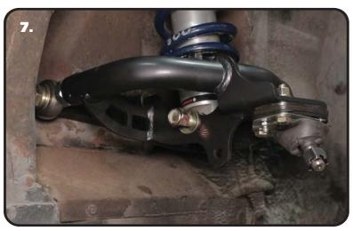
**7.** Raise the lower arm up to the CoilOver. The coilover/spacers will slip between the 2 shock mounting straps of the control arm. Line up the shock mounting holes with the through holes of shock Install a 1/2" flat washer on a 1/2" x 3 1/2" hex bolt. Insert the bolt/washer in the aligned holes. Install a 1/2" flat washer and 1/2"-13 nylok nut on the threads of the bolt. Torque to 50 ftlbs.
