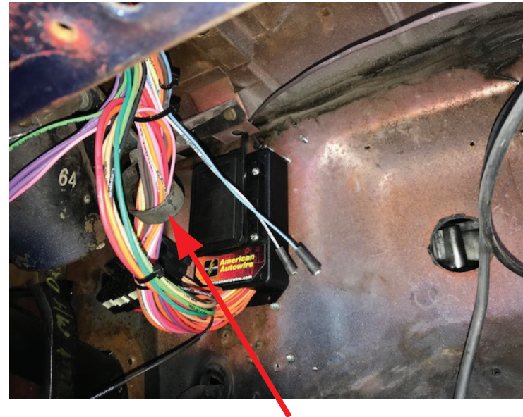
1. Mount the loaded fusebox assembly in the same general location as your original and as shown above using screws, nuts and washers "H, J and K" found in the 510472 dash loose piece kit. Route the harness up through the existing loop clamp and along the side of the wiper motor and bracket assembly.
