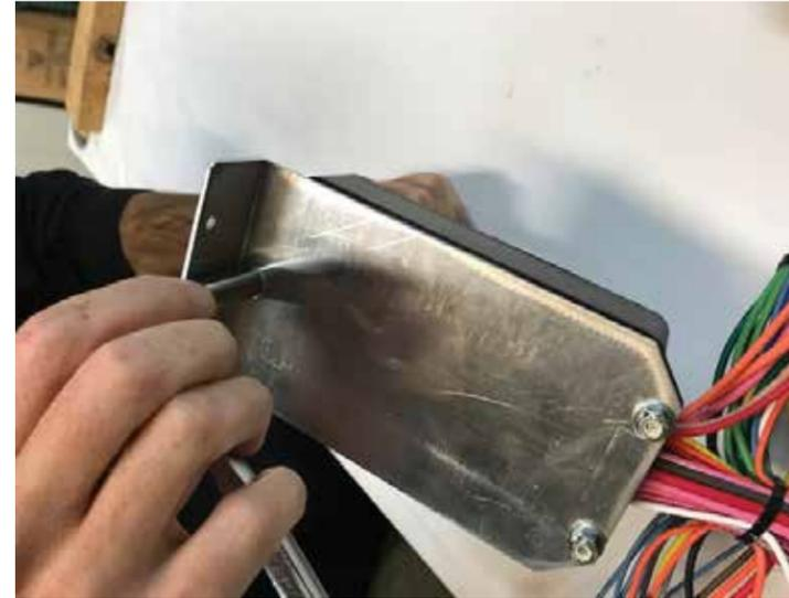
1. Assemble the mounting bracket to the fuse-loaded fusebox and harness assembly using screws, washers and nuts "H, J and K" found in the 92972060 dash loose piece kit.
