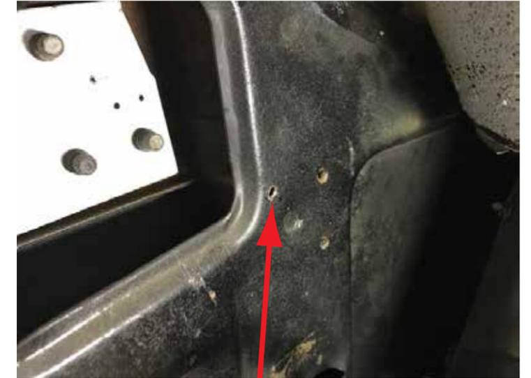
2. Using mounting template and instruction sheet 92972154, drill a new .125 mounting hole in the door hinge pillar area.
