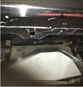
5. Install the two harness routing clips "N" into the original holes near the top of the two vertical dash supports as shown above.
