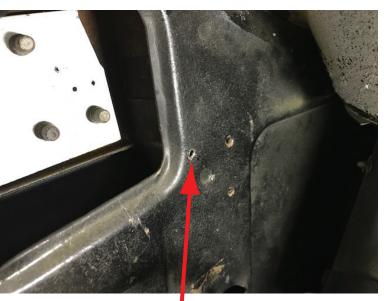
2. Using mounting template and instruction sheet 92972154, drill a new .125 mounting hole in the door hinge pillar area.
