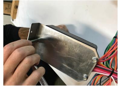
1. Assemble the mounting bracket to the fuse-loaded fusebox and harness assembly using screws, washers and nuts "H. J and K" found in the 92972060 dash loose piece kit.
