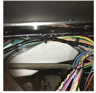
6. Snap the main harness into the two new harness routing clips "N" so that the harness routes over the cluster opening area as shown above. After you plug your wiper harness into the white AAW "wiper feed" wire from page 6, you can snap that harness into the two mounting clips as well.
