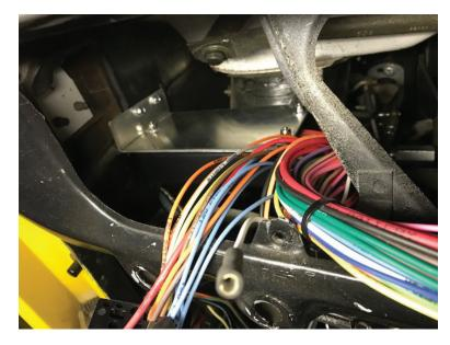
4. Tuck the "bracket, fusebox and harness assembly" down inside the dash opening, and using screws and washers "F and G" found in the 92972060 dash loose piece kit, attach the assembly to the LH door hinge pillar area. Carefully route the harness to avoid any sharp edges on the LH vertical dash support so that you do not cut or chaff any wires.
