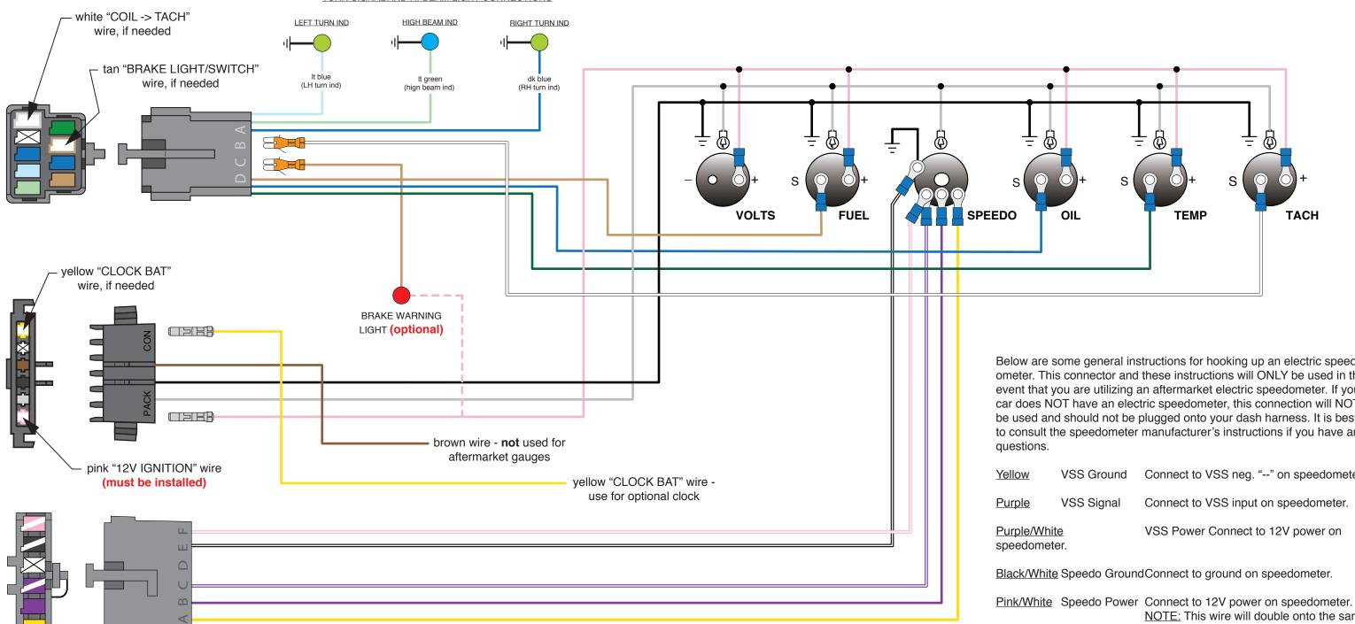
TURN SIGNAL AND HI-BEAM LIGHT CONNECTIONS
