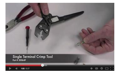
The terminals that we supply in our kits, utilize what is known as an F crimp. The F crimp, in a cross section, will look like the illustration below, when done correctly.
