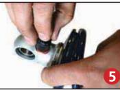
Once the knob is removed slide a Delrin washer over the eyelet. Next, slide the upper spring mount (803-00-199) over eyelet as seen in figure 4.
