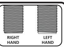
THE 4-LINK BARS, R-JOINTS, AND JAM NUTS HAVE RIGHT HAND AND LEFT HAND THREADS. THIS ALLOWS THE BAR TO BE ADJUSTED WITHOUT REMOVING IT. THE HEX END OF THE BAR IS LEFT HAND THREAD. THE LEFT HAND JAM NUT HAS AN COUNTER-CLOCKWISE ARROW STAMPED INTO IT. IMAGE 3 WILL HELP YOU DETERMINE THE THREADS OF THE R-JOINTS.
