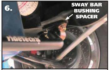
**6.** Install a 3/8" flat washer on each of the (4) 3/8" x 1 1/2" bolts. The sway bar bushing spacer will be installed between the sway bar bushing and frame. Push the bar up to the frame, installing the spacer in place. Hold it in position and install (2) bolt/washers in each side. Install a 3/8" flat washer & 3/8" nylok nut on the bolts and snug the hardware.
