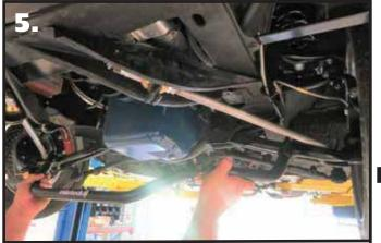
**5.** Install the sway bar in position in the car. The center of the bar should be to the front of the car. The outer arms of the sway bar will bend upward. Use **Picture 6** as a reference.
