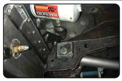
**8.** Eccentric eliminator plates are included, one must be installed on each side of the frame. Start out with it in the center, make sure both plates are in the same position. Attach the other end of the lower control arm to the factory frame mount using a  $\frac{1}{2}$ " x 4  $\frac{1}{2}$ " bolt and Hex nut. Torque to 50 ft-lbs. Install the grease zerk in the control arm sleeve.
