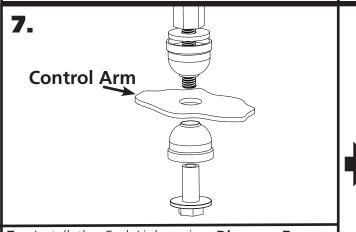
**7.** Install the End Links using **Diagram 7** as a reference. Tighten the end link barrel nut until it is flush with the end of the bolt, and then tighten it 2 more complete rounds.
